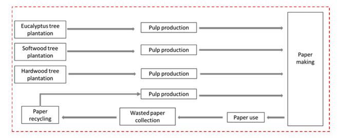
**Figure 1.** Scheme of conventional paper production system. The system boundary is represented by the dashed line and transport phases are represented by grey arrows.
