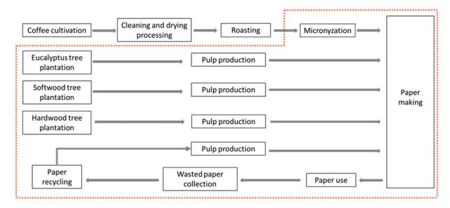
**Figure 2.** Scheme of the paper production system using coffee silverskin as raw material. The system boundary for silverskin as a byproduct of coffee roasting is represented by the dotted line and transport phases are represented by the grey arrows.
