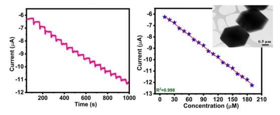
**Figure 6.** Chrono–amperometric response (left) of N-Co-MOF/GCE for the successive addition of 10  $\mu$ M of H<sub>2</sub>O<sub>2</sub> in 0.1 M PBS (pH = 7) under constant stirring, -0.35 V. To the right, the figure shows the change in current at different concentrations of H<sub>2</sub>O<sub>2</sub>, the inset shows a TEM image of the Nitrogen-enriched MOF. Adapted with permission from [61].
