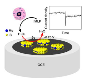
**Figure 9.** Schematic representation of a hydrogen peroxide  $H_2O_2$  biosensor based on  $MoS_2$  nanoparticles. With permission from [82].
