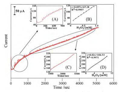
**Figure 11.** Amperometric responses of sequential additions of  $H_2O_2$  at the MWCNT–PEDOT/GCE in pH 7 PBS. Rotating speed = 2000 rpm,  $E_{app.} = -0.5$  V. The blank amperometric response of MWCNT–PEDOT/GCE is tested during 0–200 s. Inset: (**A**) scale-up amperometric response to the first  $H_2O_2$  additions; (**B**) calibration plot of  $H_2O_2$  concentration; (**C**) amperometric response to  $H_2O_2$ ; (**D**) complete calibration plot. With permission from [96].
