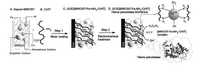
**Figure 10.** Schematic representation (**A**–**D**), of the construction of a chemically modified vitreous carbon electrode biosensor of impure multi-walled carbon nanotubes (MWCNT-Fe)-chitosan biopolymer (H<sub>2</sub>N-CHIT) (GCE/[MWCNT-Fe:H<sub>2</sub>N-CHIT]) for the electrocatalytic and electrochemical detection of hydrogen peroxide (H<sub>2</sub>O<sub>2</sub>) in phosphate buffer (PBS) pH 7. With permission from [95].
