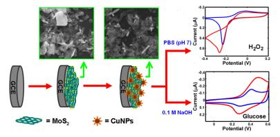
**Figure 8.** Modified glassy carbon electrode made of multilayer Cu/molybdenum disulfide (CuNFs-MoS<sub>2</sub>/GCE) with 3D nano-flower shape for non-enzymatic sensing. (**Left**) schematic representation of the fabrication of the CuNFs-MoS<sub>2</sub>/GCE, and (**Right**) possible reaction mechanisms at the electrode during the analysis for  $H_2O_2$  and glucose. With permission from [81].
