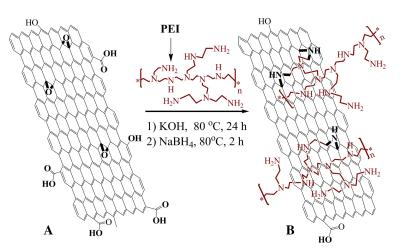
**Figure 12.** Schematic representation of the functionalization of graphene. (**A**) graphene oxide sheet; (**B**) PEI-functionalized graphene. This composite was prepared firstly by stirring PEI and graphene in KOH at 80 °C during 24 h. Then, NaBH<sub>4</sub> was added to the mixture and kept at 80 °C for 2 h. The PEI-functionalized graphene was collected by centrifugation and wash with distilled water. With permission from [97].
