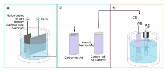
**Figure 5.** A general scheme for the synthesis of silver particles (**a**), their immobilization on the carbon rod electrode (**b**), and electrode utilization as a  $H_2O_2$  sensor (**c**). With permission from [55].
