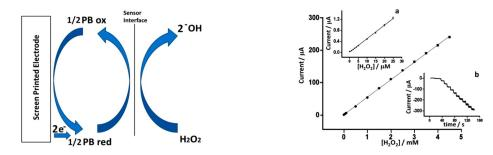
**Figure 3.** Electrochemical characterization of the electrodes with electrodeposited Prussian blue nanoparticles (PBNPs) layers. (**Left**) mechanism of the catalytic  $H_2O_2$  reduction mediated by Prussian blue (PB), (**Right**) calibration curve of  $H_2O_2$  on PBNP screen printed electrodes (SPEs). (**a**) Detail in the concentration range between 0 and 25  $\mu$ M and (**b**) raw amperometric data from 0 to 4.5 mM. With permission from [29].
