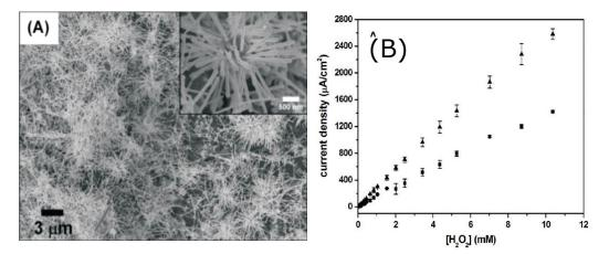
**Figure 4.** (**A**) SEM image of Ag urchin-like NWs on an SPC electrode (inset: enlarged view of a single cluster of urchin-like Ag NWs; (**B**) calibration curves of amperometric tests. Adapted with permission from [9].
