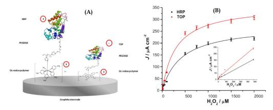
**Figure 14.** (A) Schematic representation of the biosensor based on HRP and the one based on TOP enzymes; (B) calibration curves for both biosensors in a FIA System with PBS buffer at pH 7 with 0.1 M KCl as carrier, and 20  $\mu$ L sample injection volume, -0.1 V vs. Ag | AgCl (0.1 M KCl). The inset shows the linear section of the curves. With permission from [110].
