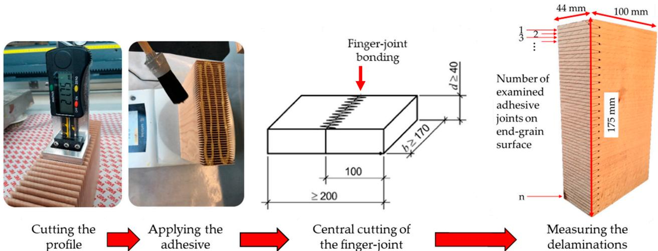
**Figure 3.** Manufacturing of delamination specimens and adhesive joints examined on the end-grain surface, technical drawing from [4] was adapted for this figure.
