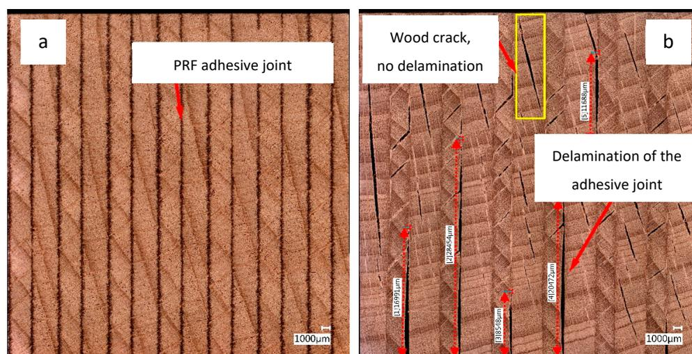
**Figure 8.** Delamination specimen before (a) and after (b) the delamination test according to [4], images taken with digital microscope VHX-5000 (Keyence, Osaka, Japan).
