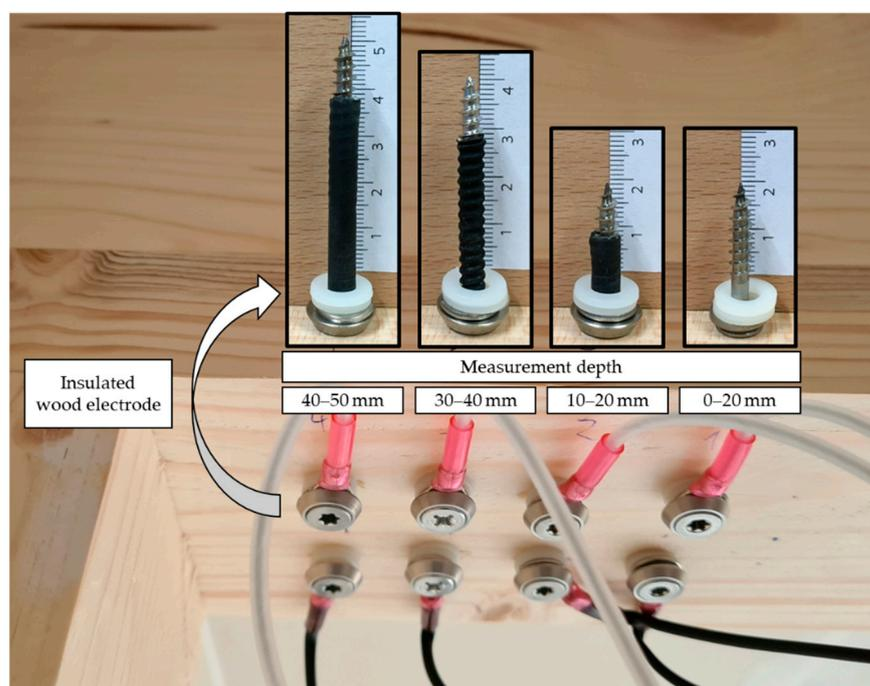
**Figure 2.** Resistance-based measurement of the wood moisture content of the beech glulam at different measuring depths.
