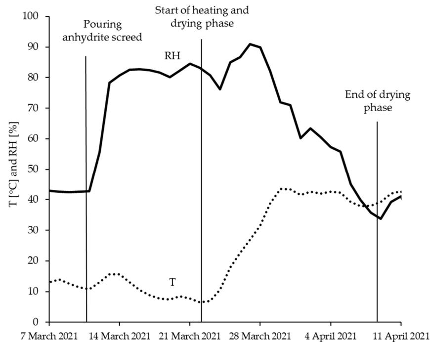
**Figure 5.** Course of temperature (T) and relative humidity (RH) in the test building during the monitoring experiment of the beech glulam.
