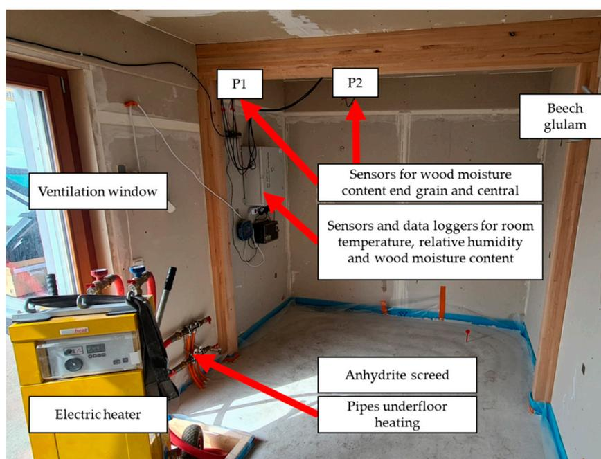
**Figure 1.** Monitoring experiment of beech glulam in the test building and positions of the measurement equipment.
