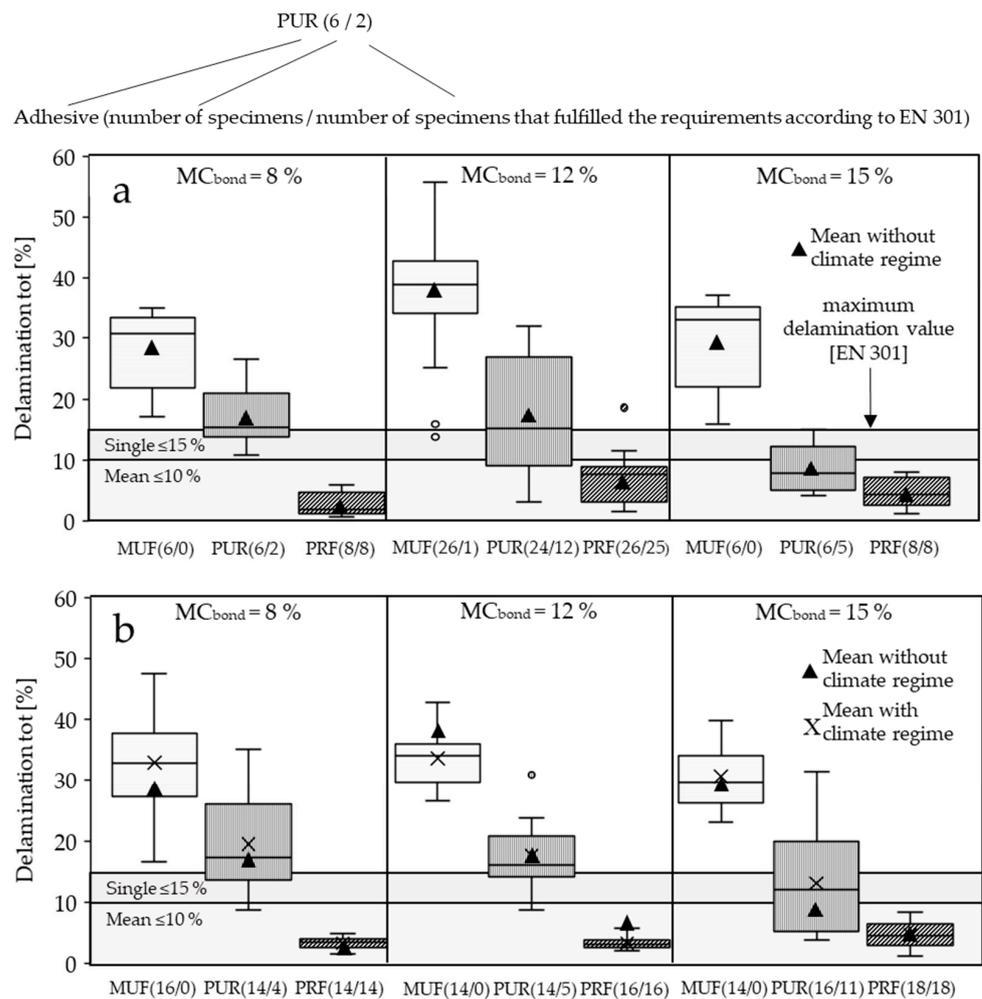
**Figure 7.** Delamination resistance of beech finger-joints depending on adhesive system and bonding wood moisture content ( $MC_{bond}$ ) according to different test methods: (a) = Delamination test without alternating climate regime, (b) = Delamination test with previous alternating climate regime.
