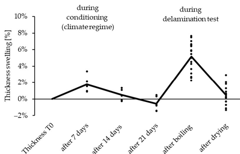
**Figure 9.** Change in specimen thickness during alternating climate regime and delamination testing.
