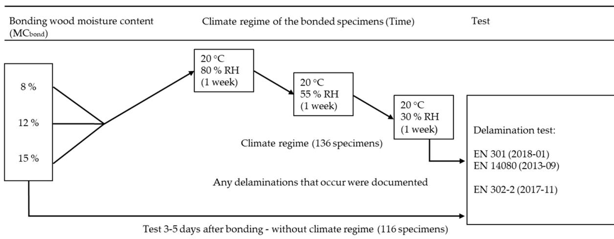
**Figure 4.** Course of the delamination test without and with previous alternating climate regime (RH = relative humidity).
