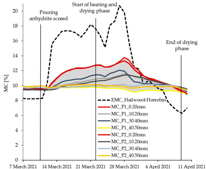
**Figure 6.** Wood moisture content (MC) of beech glulam at different measuring depths during monitoring experiment and calculated wood equilibrium moisture content ( $EMC_{calc}$ ) resulting from the climatic conditions in the test building; measured values were temperature (T)-compensated and normalised.
