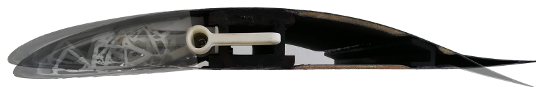
Figure 12. Morphing wing demonstrator based on topology optimization results showing undeformed and deformed states.
