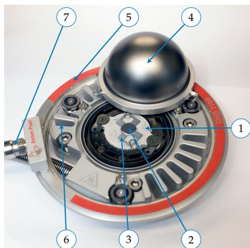
**Figure 2.** Image of the DOMED HOT STAGE: (1) AlN base plate; (2) sample; (3) TiAl holders; (4) graphite dome; (5) ring with cooling air exhausts; (6) heat sink; (7) feed pipes.
