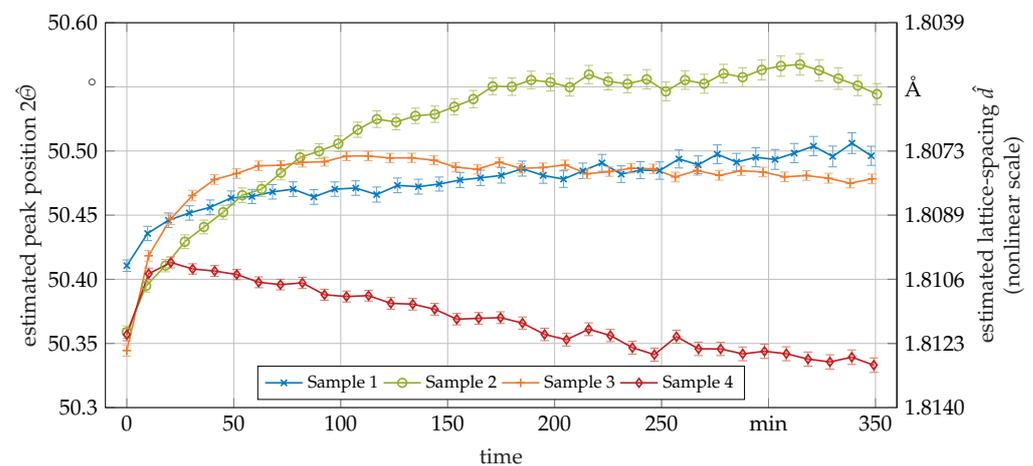
**Figure 11.** XRD based estimation of peak positions  $2\hat{\theta}$  of the (002)- $\gamma$ -peak over the time spent in the HT measured in situ. The estimated lattice spacing was calculated using the Bragg equation. Error bars are related to the  $2\hat{\theta}$ -scale.
