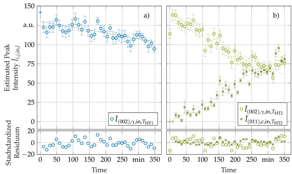
**Figure 8.** Estimated peak intensities  $\hat{I}_{i,j,in,l}$  as acquired by fitting Voigt-functions to the in-situ datasets recorded during HT with XRD of (a) sample 1 at  $T_{HT1}$  ( $T_S \approx 644^\circ\text{C}$ ) and (b) sample 2 at  $T_{HT2}$  ( $T_S \approx 732^\circ\text{C}$ ). Additionally given: Graph of the linear model fitted to the estimated peak intensities with smaller marks indicating datapoints excluded from the fit.
