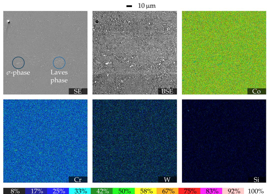
**Figure 7.** SEM images, measured with secondary electron (SE) and backscattered electron (BSE) detectors, as well as quantitative maps acquired with EDS of the bulk in sample 4 after HT with  $T_{HT4}$  ( $T_S \approx 908^\circ\text{C}$ ). Spotty dots: Laves-phase; Light gray patches:  $\sigma$ -phase.
