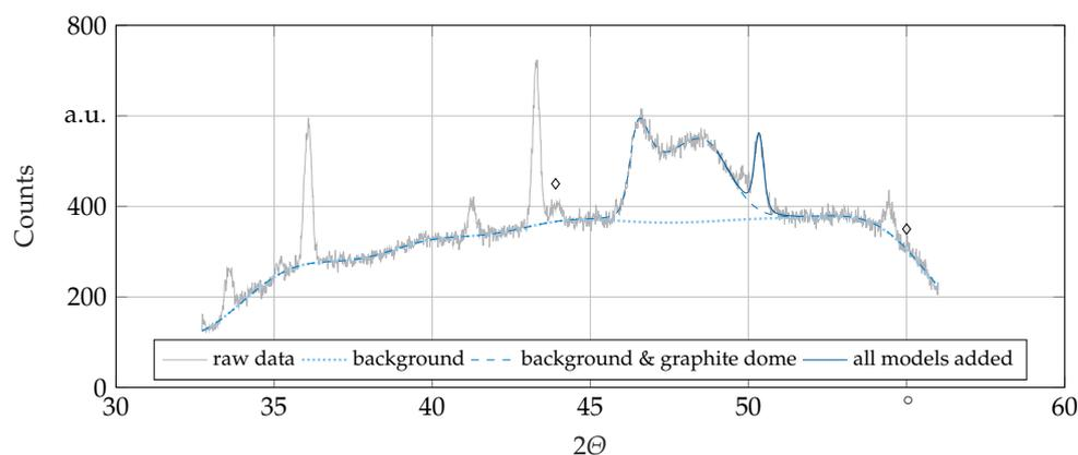
**Figure 3.** Diffractogram of the last frame of the in-situ dataset from sample 4 at  $T_{TH4}$  with graphs of the various models fitted to the raw data. Diamond markers: Possible peaks of a high temperature phase not present in ambient conditions.
