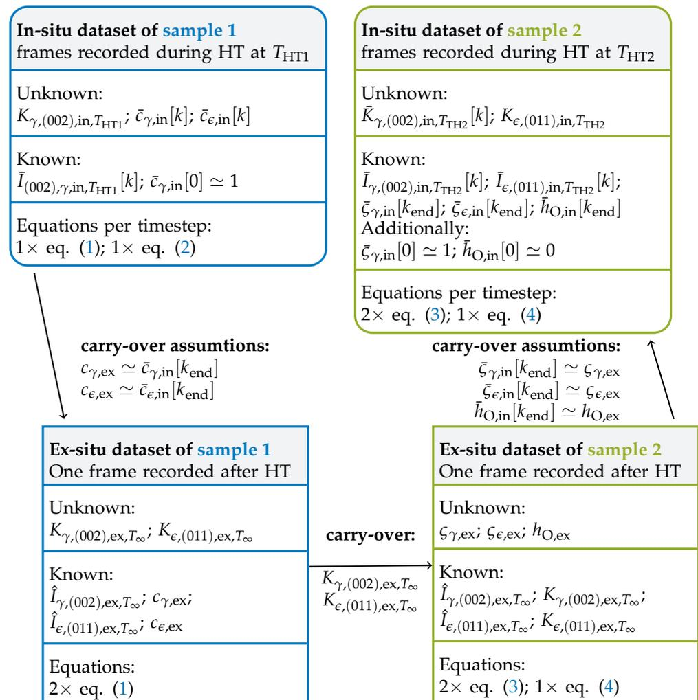
**Figure 4.** Flow chart for the calculation of calibration constants for all phases present in samples 1 and 2.
