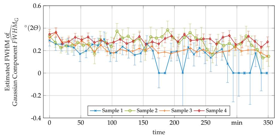
**Figure A1.** Estimated FWHM of the Gaussian component  $\widehat{FWHM}_G$  of the used Voigt peak shape function fitted to the (002)- $\gamma$ -peak over the time spent in the HT measured with in-situ XRD.
