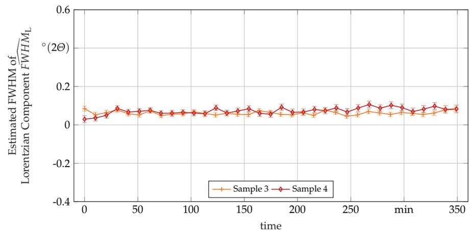
**Figure A4.** Estimated FWHM of the Lorentzian component  $\widehat{FWHM}_L$  of the used Voigt peak shape function fitted to the (111)- $\gamma$ -peak over the time spent in the HT measured with in-situ XRD. Values for samples 1 and 2 could not be given due to peak overlap with (002)- $\epsilon$ -peak.
