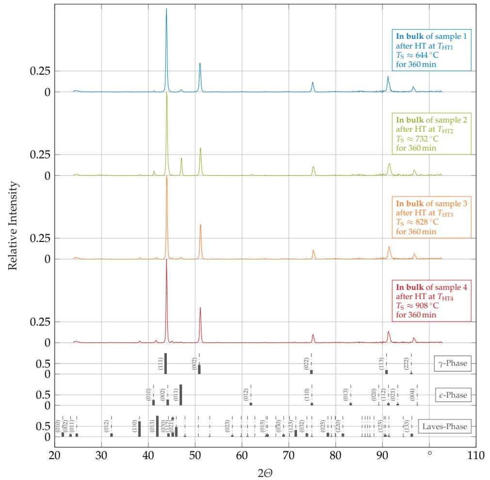
**Figure 6.** In color: Ex-situ XRD diffractograms, with intensities normalized to the highest peak in the respective pattern, of samples composed of a Co-Cr-W alloy in states AB by L-PBF and after HTs measured on the samples' bulk. Additionally in grey: Stick reference pattern calculated with VESTA [32] of a solution of W in Co fcc  $\gamma$ -phase (COD:1524796 [33]), a solution of W in Co hcp  $\epsilon$ -phase (COD:1524797 [33]), and a  $W_2Co_3Si$  Laves-phase [37].
