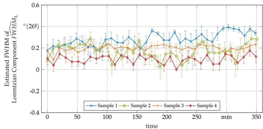
**Figure A2.** Estimated FWHM of the Lorentzian component  $\widehat{FWHM}_L$  of the used Voigt peak shape function fitted to the (002)- $\gamma$ -peak over the time spent in the HT measured with in-situ XRD.
