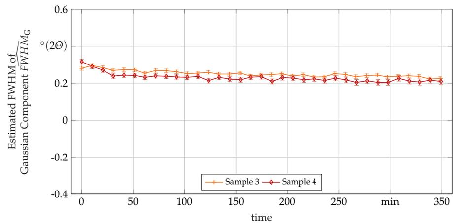
**Figure A3.** Estimated FWHM of the Gaussian component  $\widehat{FWHM}_G$  of the used Voigt peak shape function fitted to the (111)- $\gamma$ -peak over the time spent in the HT measured with in-situ XRD. Values for samples 1 and 2 could not be given due to peak overlap with (002)- $\epsilon$ -peak.
