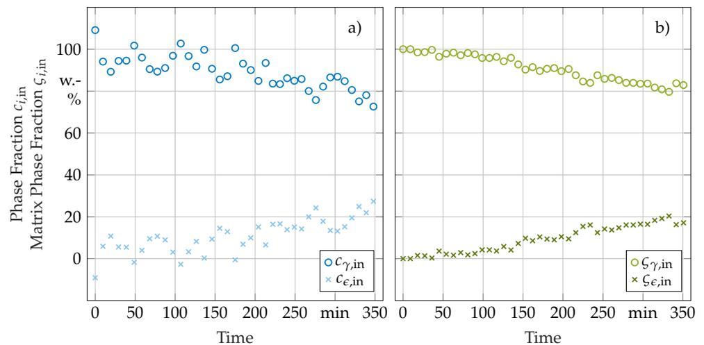
**Figure 9.** Calculated weight fractions  $c_{i,in}$  and weight fractions relative to the matrix phases  $\zeta_{i,in}$  over the time spent in the HT based on the in-situ XRD measurements for (a) sample 1 and (b) sample 2.
