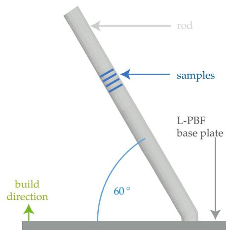
**Figure 1.** Illustration of the orientation of the samples in the L-PBF process.
