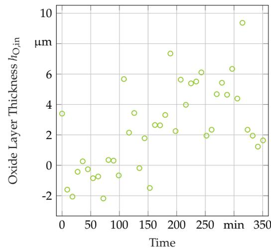
**Figure 10.** Calculated oxide layer thickness  $h_{O,in}$  over the time spent in the HT for sample 2 based on in-situ XRD measurements.
