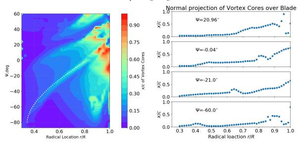
**Figure 9. Left:** Location of the vortex cores over the blade in radical region  $r/R=0.3\sim 1.0$  evolving along azimuth. Dotted line is a curve  $r/R=1/2\times 0.248\Delta\Psi^2+0.16\cos(\Psi)\Delta\Psi+0.3426$ ,  $\Delta\Psi$  in rad. **Right:** Projection of vortex cores on the blade upper surface at selected azimuths.
