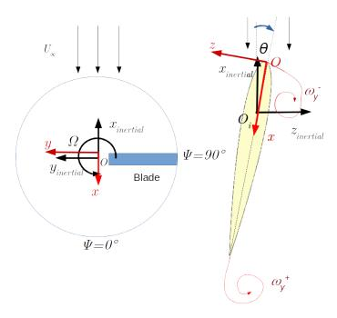
**Figure 3.** Illustration of coordinate systems used in analysis: the Inertial coordinate, of which the origin is positioned at blade rotation/pitch center, and the body-fixed coordinate, of which the origin is at blade leading edge. All of the aerodynamic variables are defined according to the body-fixed coordinate.
