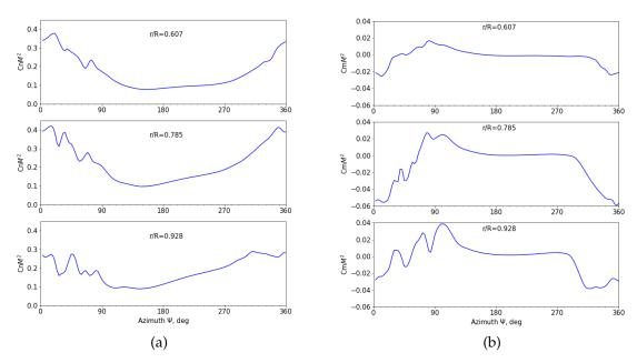
**Figure 5.** Sectional force coefficients at selected radial locations, r/R = 0.607, 0.785 and 0.928. (a): sectional normal force coefficient  $CnM^2$ ; (b): sectional pitch moment coefficient  $CmM^2$ .
