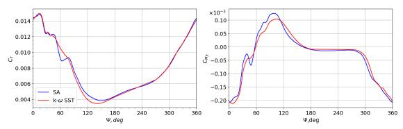
**Figure 4.** Comparison of thrust and pitching moment coefficients of the blade within one revolution by different turbulence models: Spalart–Allmaras (SA) and the  $k-\omega$  SST turbulence model.
