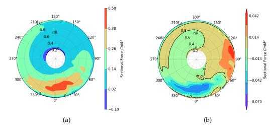
**Figure 6.** Rotor map of sectional force coefficients. (a):  $CnM^2$  sectional normal force coefficient normalised by sonic speed; (b):  $CmM^2$  sectional pitch moment coefficient.
