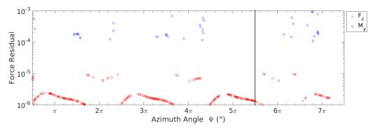
Figure 2. Force residual as a function of simulation time history expressed in azimuth angles.
