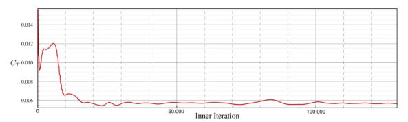
Figure A4. Thrust coefficient along inner iterations.
