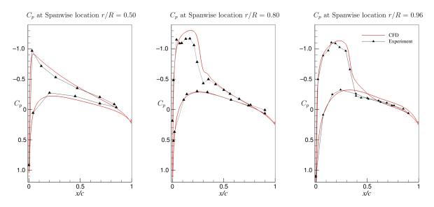
**Figure A5.** Pressure coefficient at different span-wise locations on the blade: comparison between numerical simulation with Spalart–Allmaras turbulence model and experiment result [37]).
