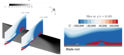
**Figure 11.** The swell structure on the blade, represented with x and y slices. **Left**: slices at r/R = 0.488 and 0.625; **Right**: slice at x/c = 0.183.
