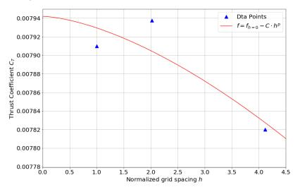
Figure A1. Grid convergence study with coarse, medium, and fine grids.
