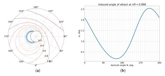
**Figure 21.** Induced AoA according to BEMT,  $\alpha_i = V_i/U(r, \Psi)$ ; (a) rotor map of  $\alpha_i$ ; (b)  $\alpha_i$  at r/R = 0.898.
