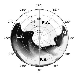
**Figure 16.** Rotor map of separation regions. F.A. is the fully attached region; L.S. is the leading edge separated region, where the LEV is attached, representing as the conical vortex structure on the rotating blade; F.S is the fully separated region due to the shedding of DSV; SI is the shock induced separation region.
