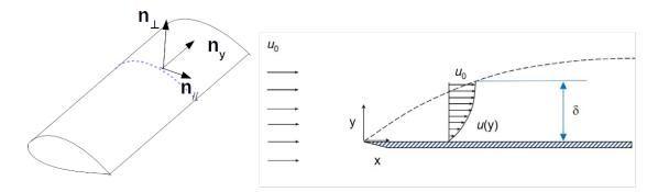
**Figure 17. left**: Illustration of coordinate system used to post-process shape factor; **right**: schematics of boundary layer over a flat plate.
