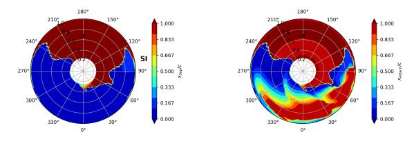
**Figure 14.** Rotor map of chord-wise separation  $x_{Sep}/c$  and attachment  $x_{Attach}/c$  locations. The direction of the free stream is from  $\Psi = 180^{\circ}$  to  $\Psi = 0^{\circ}$ , and the rotating direction is counterclockwise.
