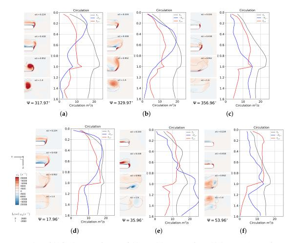
**Figure 10.** Snapshots of the flood contour of vorticity field  $\omega_x$  and the contour of  $\omega_y$  in blade tip area (0.94 < r/R < 1.125) at different chord-wise sections; The circulation  $\Gamma_{i\pm} = \int \int_S \pm \omega_i dA$ , where S is the tip region where  $\omega_x > 0$ , i = (x, y). Azimuth positions:  $\Psi = (\mathbf{a}) 318^\circ$ ; (**b**)  $330^\circ$ ; (**c**)  $357^\circ$ ; (**d**)  $18^\circ$ ; (**e**)  $36^\circ$ ; (**f**)  $54^\circ$ .
