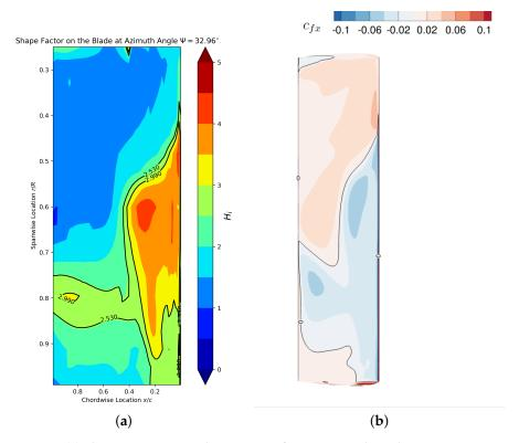
**Figure 18.** (a) Shape Factor  $H_i$  on the upper surface at azimuth angle  $\Psi = 32.9^{\circ}$ , two contour lines indicate the upper and lower bound of  $H_i$  value to determine the separation; (b) skin friction  $c_{fx}$  on the upper surface at azimuth angle  $\Psi = 32.9^{\circ}$ , the 0 contour line showing the separation line.
