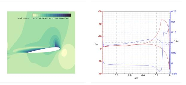
**Figure 15.** Mach contour of the slice r/R = 0.898 and the corresponding pressure coefficient  $c_p$ , skin-friction in the x-direction  $c_{fx}$  on the blade section, azimuth angle  $\Psi = 90^{\circ}$ . On the upper surface,  $c_{fx}$  drops from positive to negative and crosses 0 at x/c = 0.12, where the  $c_p$  shows a sharp increase.
