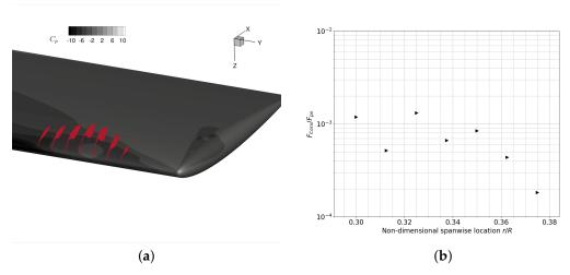
**Figure 12.** Comparison of the pressure force and the Coriolis force in vortex cores. (**a**) area of integration, where Q > 0; (**b**) ratio of Coriolis force in the *x*-direction and pressure force in the *x*-direction  $\Delta F_{Cor}/\Delta F_{px}$ .
