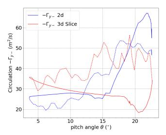
**Figure 20.** Vorticity strength of the counter-clockwise vortex over the upper surface of the pitching airfoil and the slice of the rotating blade, with solid lines representing the upward pitching and dashed lines the downward pitching. The circulation  $\Gamma_{V-} = \iint_S \omega_V^- dA$ , and in region S, Q > 0.
