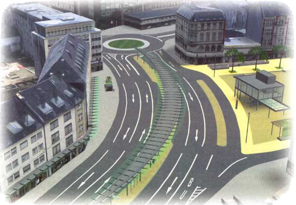
Figure 1. Integration of 3D CAAD and GIS models in an urban planning scenario. Whereas architecture models provide detailed information about the planned objects, GIS models set the environmental context. Image: City of Solingen, Stadtdienst 621/623. Planning version for the rebuilding of the Graf-Wilhelm-Platz. Design by Quick / Beckmann / Quick Architects, Berlin
