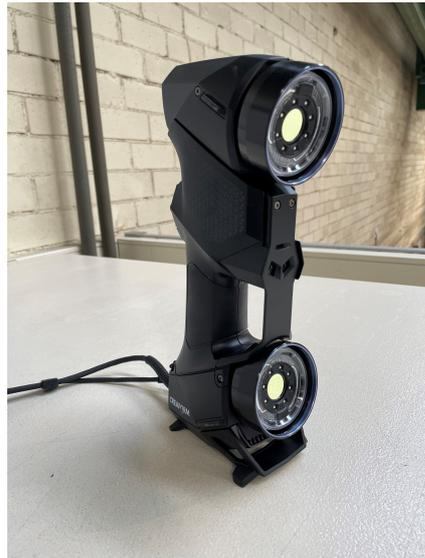
**Figure 3.** Three-dimensional (3D) laser scanner used for the measurement of displacements of the samples during the cyclical freeze–thaw temperature load.
