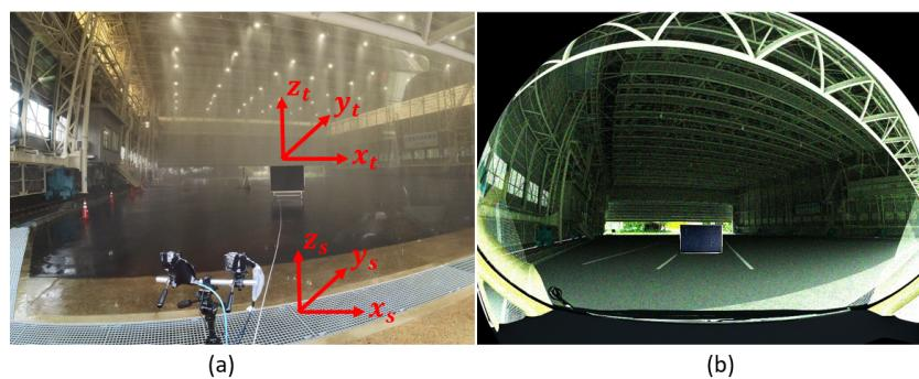
**Figure 6.** (a) Real setup to validate the time domain and point cloud data. (b) Static simulation scene to validate the time domain and point cloud data. The 3%-reflective target with an area of  $1.3 \text{ m} \times 1.3 \text{ m}$  was placed in front of the sensor at different distances. The actual and the simulated sensor and target coordinates are the same. The ground truth distance  $d_{GT}$  is calculated from the sensor's origin to the target's center.
