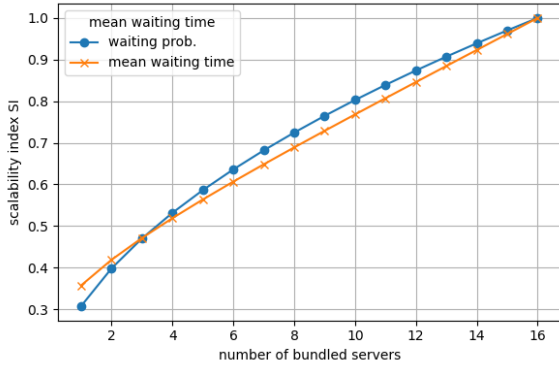
FIGURE 13: Economies of scales of the IoT load balancer – The scalability analysis uses as reference system an M/M/16 waiting queue with n processing units, service rate \mu per unit, arrival rate n\lambda . As target measure, the waiting probability and the expected waiting time are considered. The parameter under investigation is the load over the range [0.1; 0.9] .
