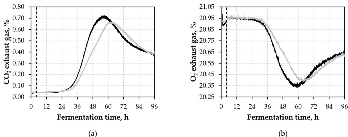
**Figure 3.** Carbon dioxide (CO<sub>2</sub>) (a) and oxygen (O<sub>2</sub>) (b) concentrations in the exhaust gases of two SSF with *A. niger* ATCC 11414  $\Delta$ *gaaX* on non-milled SBPP. The pH was buffered at pH 4.5, and the wet heap of SBPP was inoculated with  $6.25 \times 10^6$  spores per L. The aeration was started with  $1 \text{ L h}^{-1}$  of sterile air after 4 h to prevent spore loss (indicated by the dashed line).
