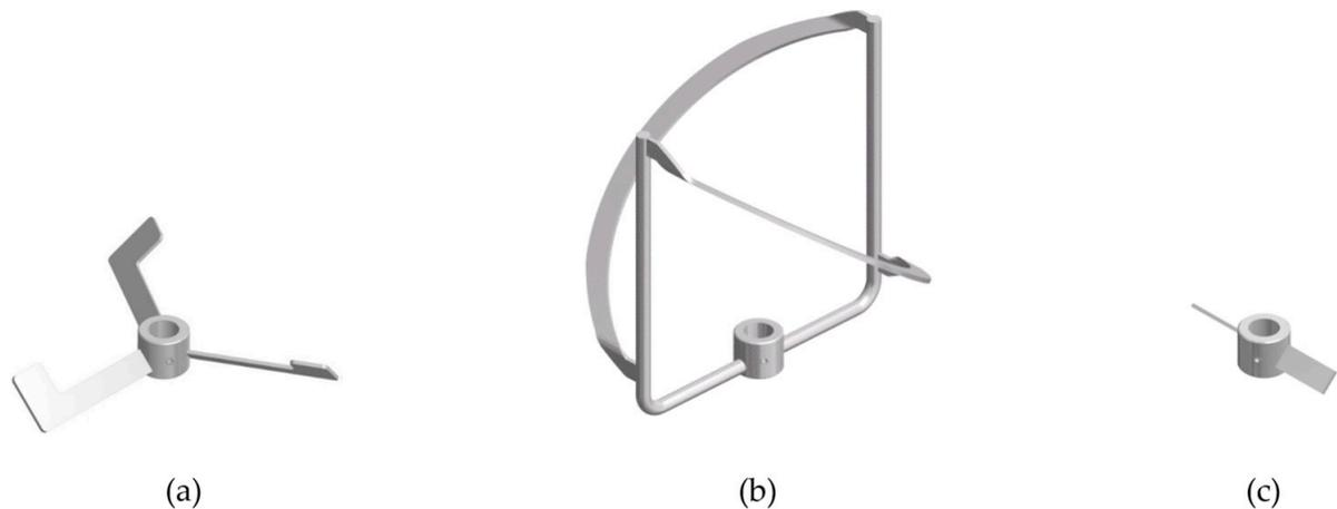
**Figure 1.** Stirrers made of steel used for SSF and subsequent hydrolysis of SBPP: (a) anchor stirrer with a maximum diameter of 14 cm and a maximum height of 2.2 cm, (b) one-fold helical stirrer with a maximum diameter of 14 cm and a maximum height of 13.5 cm, and (c) pitched-bladed impeller (45°) with a diameter of 7 cm. Stirrer figures adapted from Labfors 5 operating manual (Labfors, Infors-HT, Bottmingen, Switzerland).
