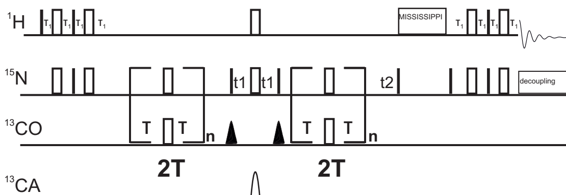
Figure 6.1: HNCO CPMG INEPT-based pulse scheme. The delays in the INEPT block were set to 2.7 msec. Filled rectangular pulses refer to \pi/2 pulses (shaped and hard) and open pulses are \pi pulses. Total mixing time during NC' correlation is equal to 4T . Similar to T_2 CPMG experiments, there is no continuous wave decoupling. Therefore, \pi pulse is set in the middle of t1 evolution. The second t2 evolution in the ^{15}\text{N} channel occurs after mixing time. It may affect the sensitivity of the experiment for low \nu_{CPMG} values.
