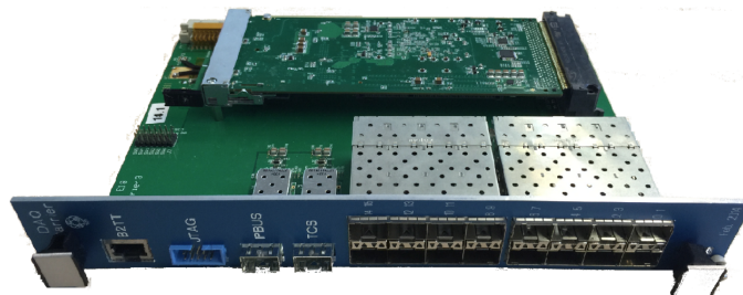
Fig. 3.8 Data Handling Card (DHC) mounted on a VME carrier card. The carrier card provides the necessary interconnection ports for the different interfaces.
