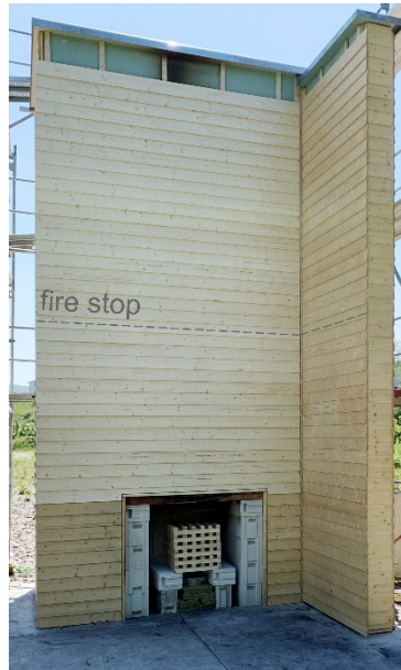
Figure PII. 7 Vertical section and photo of the façade structure with visualized fire stop in Test 1 [in mm]
