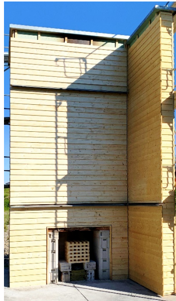
Figure PII. 7 Vertical section and photo of the façade structure with visualized fire stop in Test 1 [in mm]
