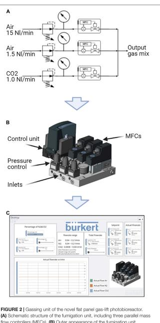
(A) Schematic structure of the fundigation unit, including three parallel mass flow controllers (MFCs). (B) Outer appearance of the fumigation unit developed in cooperation with the cooperation partner Christian Bürkert GmbH & Co. KG. (C) Overview of an exemplary user interface, which can be adjusted according to the experimental requirements. Features of the software comprise real time parameter monitoring and creation of quick access buttons.
