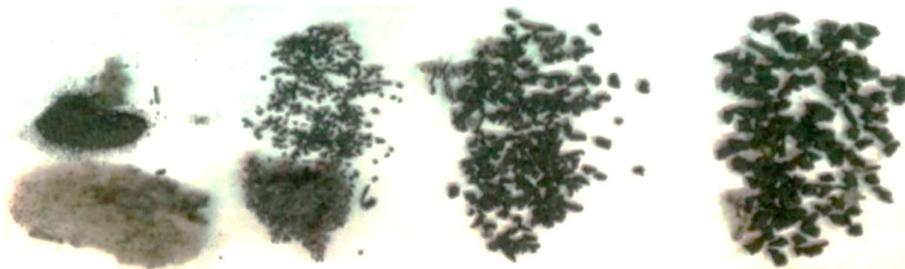
**Figure 2.** Crumb rubber manufactured via the mechanical shredding of recycled tires.
