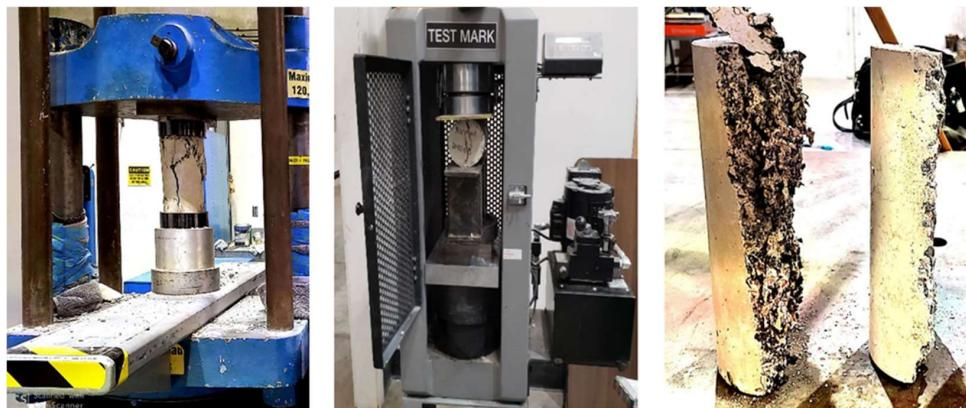
**Figure 6.** Compression test (left), splitting tensile test (middle), and broken splitting tensile samples of TDA and conventional concrete (right).
