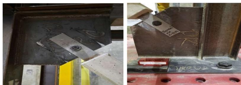
**Figure 8.** Bolted connections at the top (left image) and bottom (right image) of the brace.
