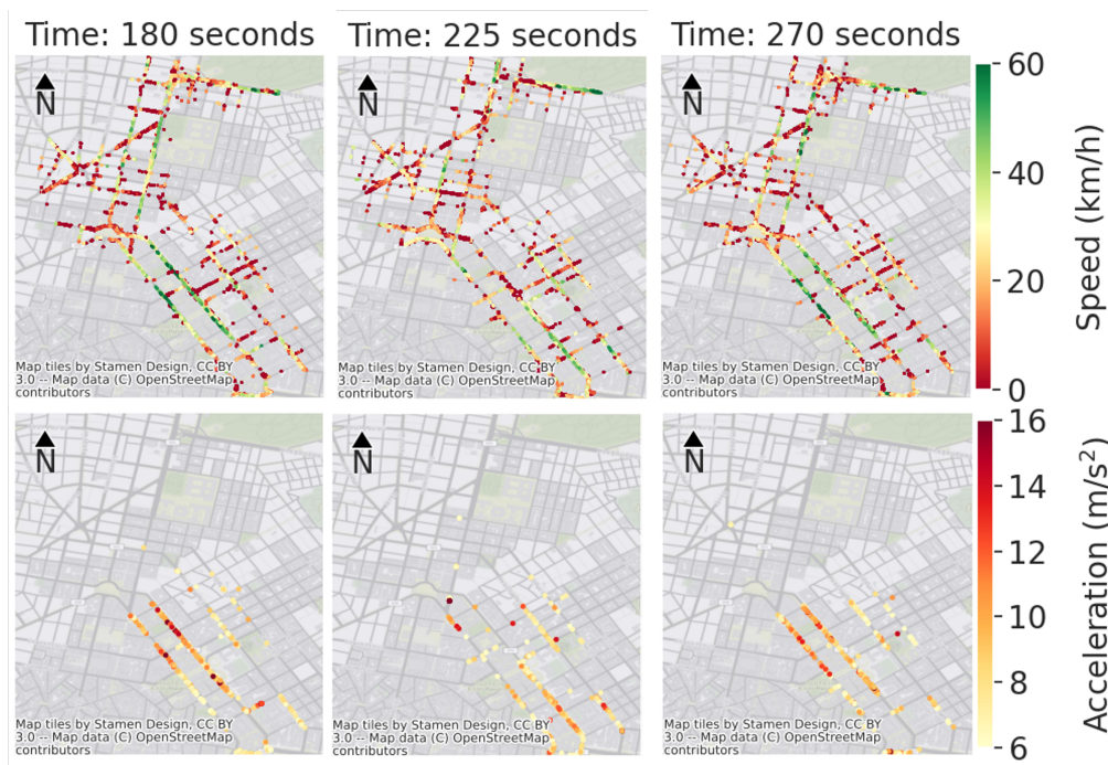
Figure 4.7: Heatmap showing location-wise speeds and accelerations (exceeding 6 \text{ m/s}^2 ) at frames 45 seconds apart to highlight the correlation between them and the periodicity of excess accelerations at about 90 seconds. Similar findings were found for deceleration. ©2023 IEEE.
