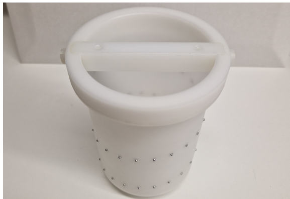
(c) Cylinder part with calibration structure (helix)
