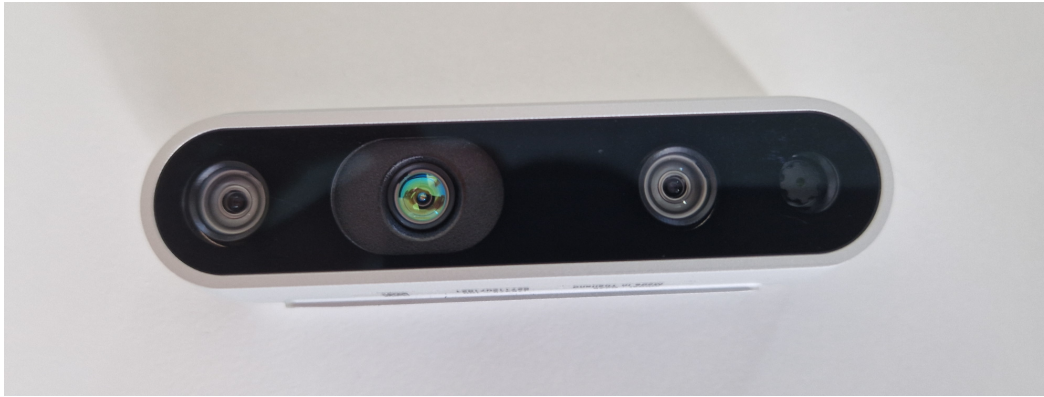
Fig. 4.5.: Intel Realsense depth camera. We used two Realsense cameras for the active collision detection algorithm described in section 4.2.3.2. The maximum resolution of the depth stream is 1280 \times 720 at 90 fps and the colored video stream has a 1920 \times 1080 resolution at 30 fps.[@Int23a]
