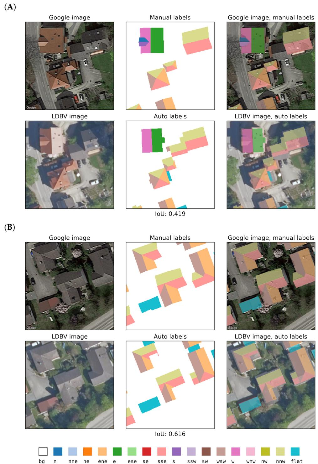
**Figure 5.** Exemplary comparison of manual and automatic samples from the small-scale datasets. IoU is given. (A) Manual labels identify dormer, auto labels do not; on the other hand, auto labels identify segments missing in manual dataset. (B) Auto labels do not cover roof overhangs and sometimes wrongly represent roof geometry, as for the cross-gabled building to the right.
