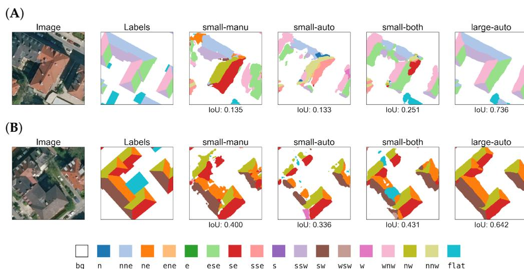
**Figure 8.** Test samples from the large-scale dataset *large-auto* at two locations (A,B), and corresponding predictions from all models. IoU with respect to labels is given for each prediction.
