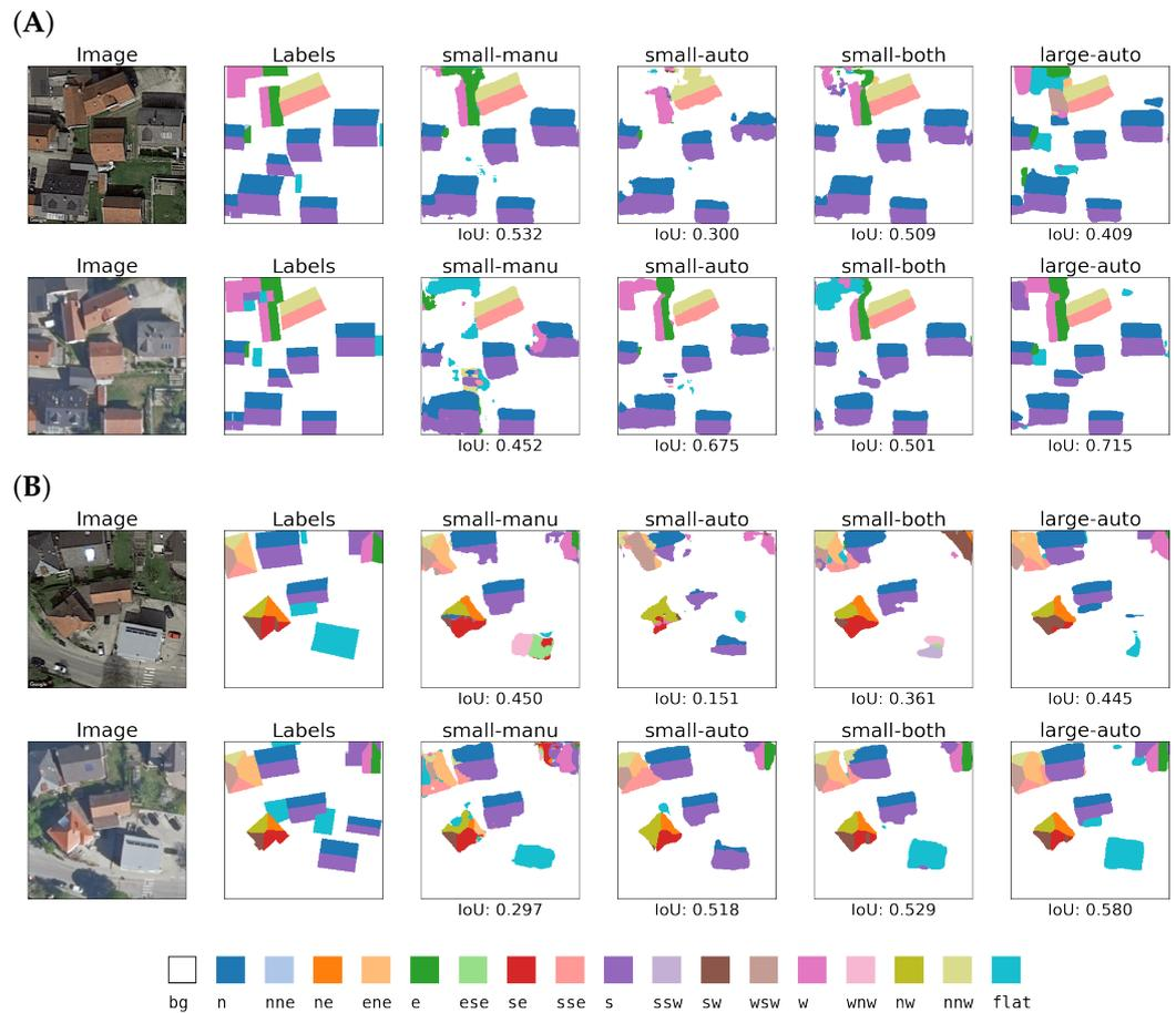
**Figure 7.** Test samples from the small-scale datasets *small-manu* and *small-auto* at two locations (A,B), and corresponding predictions from all models. For each location, the upper sample is from *small-manu* (Google image, manual labels) and the lower sample is from *small-auto* (LDBV image, auto labels). IoU with respect to labels is given for each prediction.
