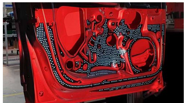
Fig. 7 Spatially dependent texture projections based on a simulated point cloud
