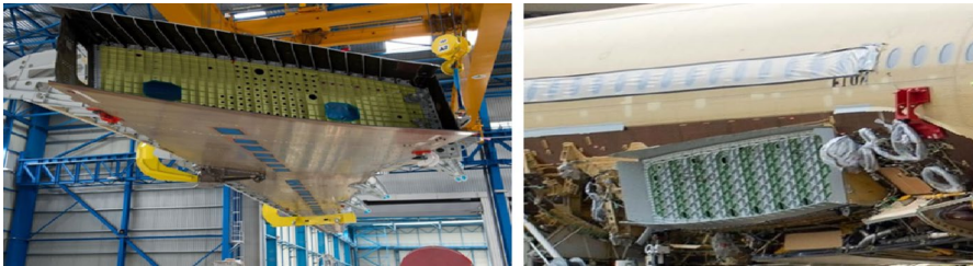
Fig. 4 Parts of wing-to-fuselage assembly for Airbus A350-900. Outer wing box (left) and central wing box (right). Photos courtesy of Airbus SAS
