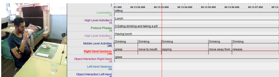
Fig. 10 Example of the annotation process. Left: a video snapshot, which is used as reference to create the annotations. Right: the corresponding annotations to the performed activity. The red vertical line indicates the time corresponding to the video snapshot
