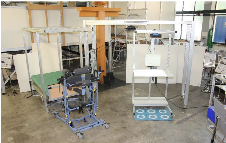
Fig. 13 The prototypes of various PI 2 Us (e.g., PI 2 U-SilverArc, PI 2 U-MiniArc, PI 2 U-SilverBed, and PI 2 U-iStander) deployed and tested in the laboratory
