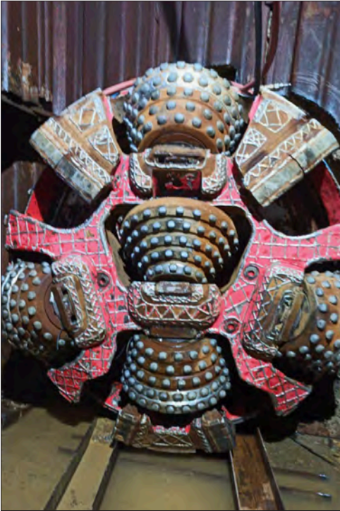
Figure 4. Cutting wheel of the AVN 800 HR after breakthrough (left) and tight jobsite installation in Hong Kong (right).
