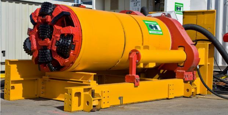
Figure 6: AVN 800 HR for hard rock with compact jacking station
