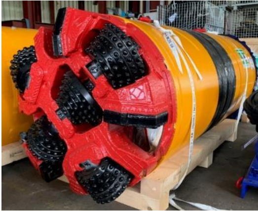
Figure 8: AVN 800 HR designed for operation in hard rock
