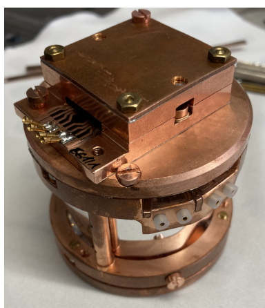
Figure 3.7: Closed detector module as it is mounted in the cryostat.
