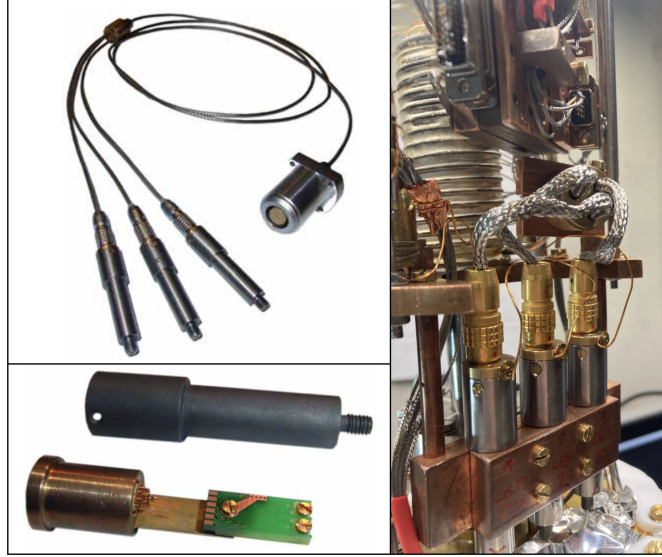
Figure 2.7: Upper left: Three channel SQUID system from Magnicon with the 300 K connector and the three SQUIDs which are located at 1.5 K. Figure adopted from [115]. Bottom left: The SQUID is encapsulated in a niobium housing (long grey cylinder). Adopted from [115]. Right: The SQUIDs are mounted on the 1 K pot stage. Additional copper strings are screwed between the 1 K pot stage and the SQUID frame for a better thermal link.
