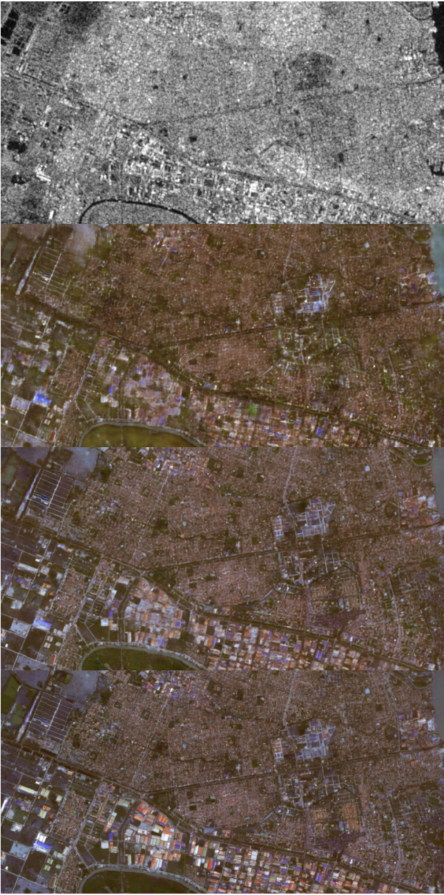
Fig. 11. Illustrations on the effect of prior guidance via SAR information. Columns: SAR input to the SAR-conditioned model, cloud-free prediction of the model conditioned on Gaussian noise, cloud-free prediction of the model conditioned on SAR information, and cloud-free observation as a reference image. The structural information provided by the SAR input provides a strong prior to the model, guiding it toward learning to remove clouds in the cloudy input time series.
