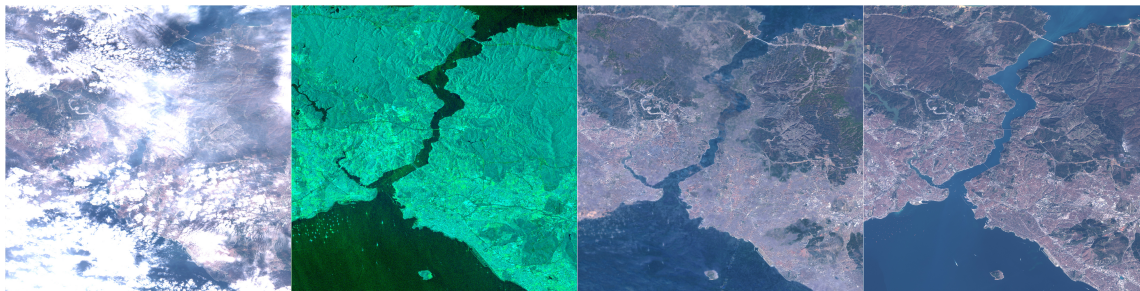
Figure 4.6: Exemplary full scene prediction. Depicted are a cloudy Sentinel-2 image, Sentinel-1 measurements, the cloud-removed prediction by DSen2-CR and a cloud-free target image of Istanbul. Despite thick cloud coverage, DSen2-CR succeeds in inferring the test scene’s structure thanks to the auxiliary radar data.
