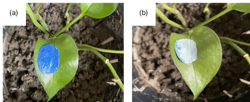
Figure 6. Photographs of the hydrogel-based detector paste on the leaves of E. aureum a) before and b) after solar radiation in a real outdoor scenario.
