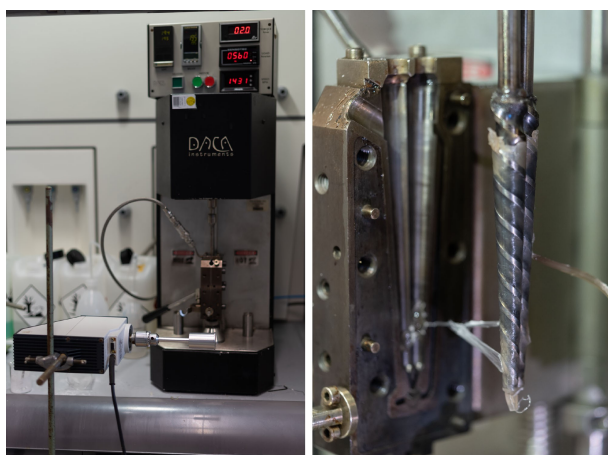
Figure 1. Set-up for fiber spinning (left) and agglutinated compounder (right) after spinning of UHMW-iPP.
