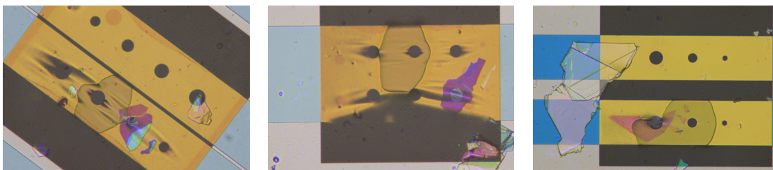
Figure 4.5: Example of a dry transfer process. Photographs of the stamping process of three different samples. During the peeling off of the PDMS, the SiN membrane and the flakes get dragged, causing the hBN and SiN membrane to buckle and wrinkle.
