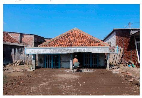
**Figure 6.** Houses with a very low roof. The landowner performs landfilling to avoid inundation, but is unable to heighten their house. Consequently, half of the house is stockpiled by the materials. Source: field data collection.
