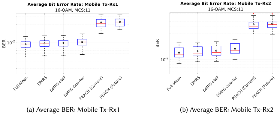
Fig. 11. Average BER for mobile Tx with 16-QAM on both receivers.
