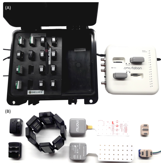
Figure 2.4: Electromyography sensors. (A) Acquisition box of Delsys (left) for the Trigno electrodes and of OTBioelettronica (right) for the MuoviPro electrodes. Both collect their electrode data via WiFi and transmit it to a computer via network cable and TCP. (B) From left to right: Delsys Trigno electrodes, Myoband from Thalmic Labs communicating directly via Bluetooth, HD-sEMG MuoviPro electrodes from OTBioelettronica, Myobock sensors from Ottobock.
