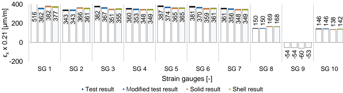
Figure 4-19: Validation for tensile load F_{max} for WP3_1.2_05 representatively for WP3_1.2
