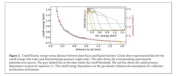
cutoff, which is defined as the energy where the signal intensity drops to 30% of its plateau value, changes with the distance between the liquid microjet and the laser focus.
