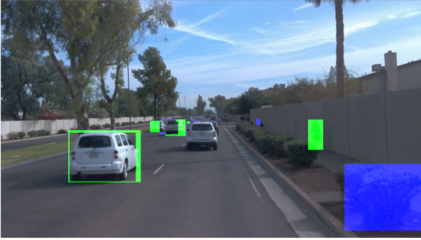
Fig. 7: Difference between the to ML approaches. Blue indicates areas detected by MobilNet only, green indicates areas detected by EfficientDet only.
