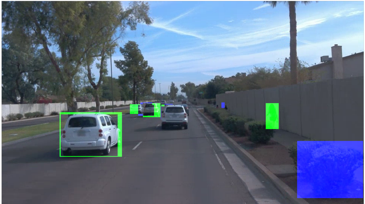
Figure 3.23: Difference between the two ML approaches. Blue indicates areas detected by MobileNet, green indicates areas detected by EfficientDet. (Source: [I], ©2022 IEEE)
