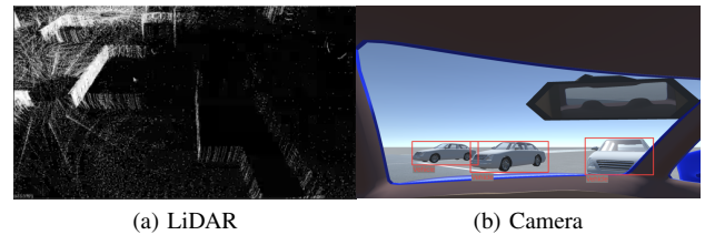
Fig. 7: LiDAR (a) and camera with object-classification (b) in OpenROUTES3D.
