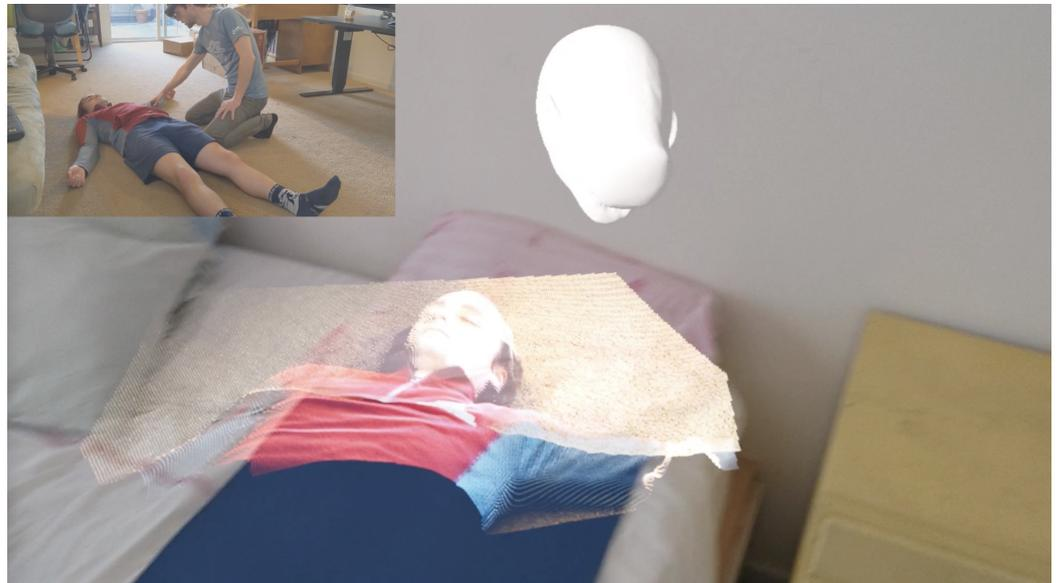
**Figure 2.** Small image top-left: A trainer (streamer) wearing a HoloLens 2 and looking at a patient. Large image right: A mixed reality capture of the student's first-person view (receiver) showing the color point cloud of the patient from the perspective of the trainer wearing the HoloLens 2. The white head model represents the head pose of the trainer. A full (video demo, <https://youtu.be/oo6A1yKrJFY>, accessed on 22 February 2022) also shows the segmentation of the patient.
