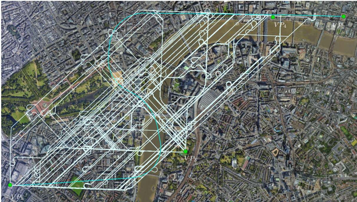
Figure A-4: A top view of an alternative path (cyan) in the trajectory tree \mathcal{T}_{2,2} and respective CSFL solution (white) with \Delta t_C = 30s . 439 alternate trajectories are planned to alternate vertiports VP_1 , VP_3 and VP_4 . The London Eye ferris wheel and several high-rise building along the river are obstacles across all flight levels.
