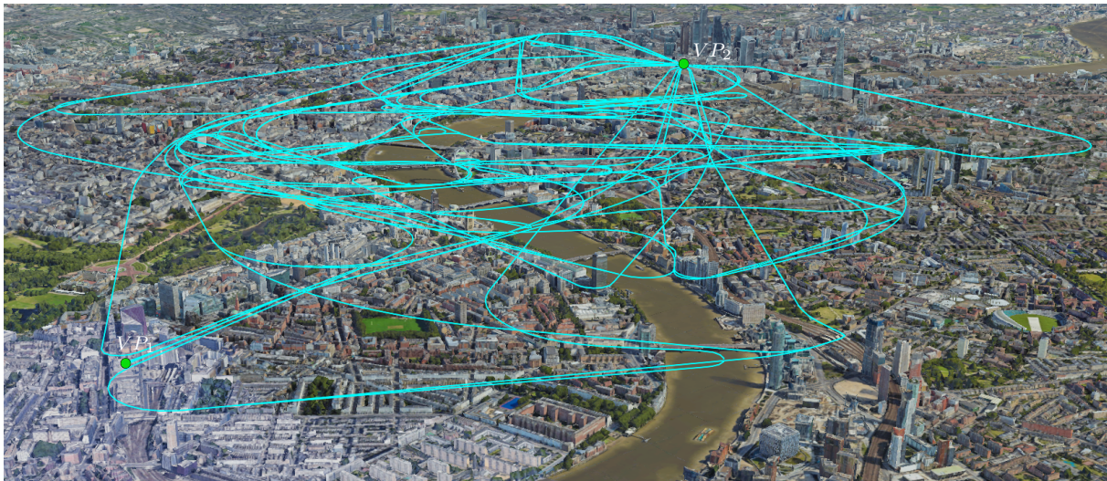
Figure A-2: A three-dimensional perspective of the trajectory tree \mathcal{T}_{2,2} . It can be observed, how trajectories descend into vertiport VP_2 on the approach funnel.
