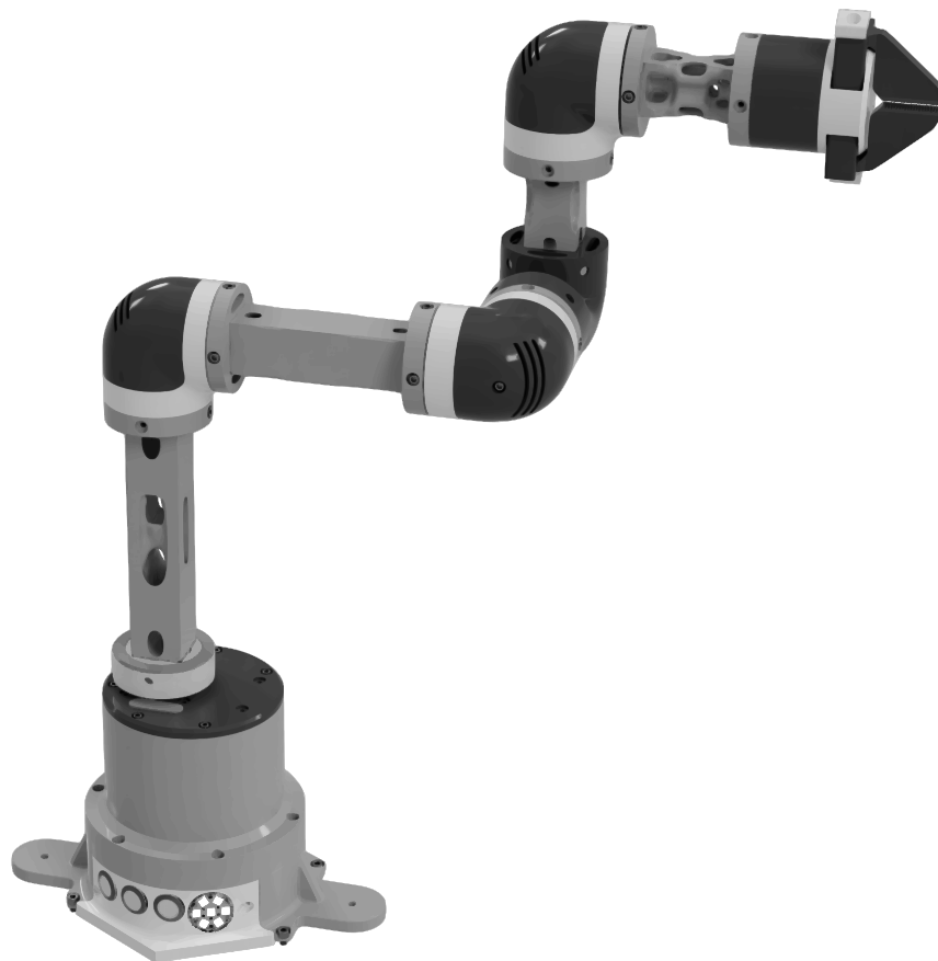
Figure 6.18: Resulting low-cost lightweight robot with topology optimized and post-processed structural elements for n_p=100 load cases
