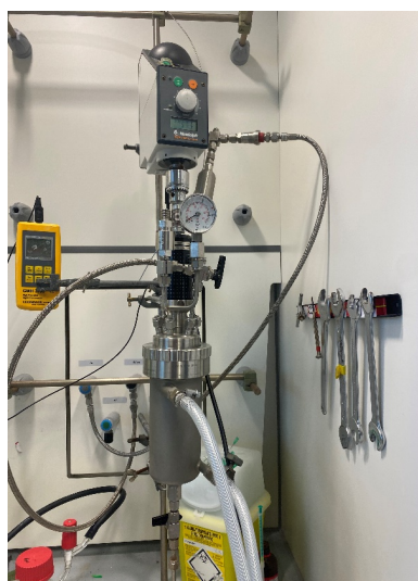
Figure S16. Photograph of a 250 mL double-walled Büchi steel autoclave used for polymerization up-scaling.
