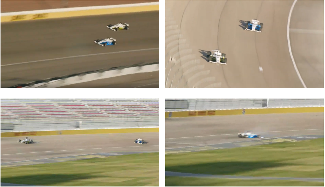
Figure 18: The final overtake in the final of the Autonomous Challenge at Las Vegas Motor Speedway and spin-out of the TUM vehicle at 250 \text{ km h}^{-1} . Image credits: Indy Autonomous Challenge. Full video available at [33].
