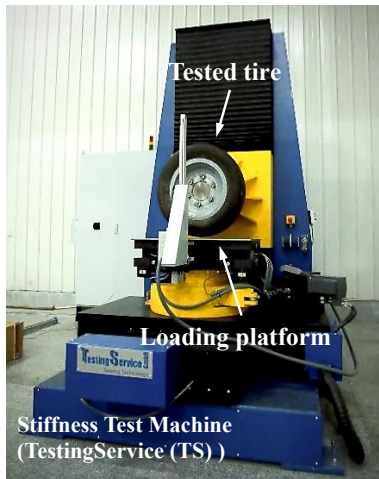
(a) System implementation of the stiffness test machine with a measured tire.
