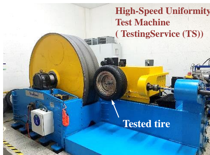
Figure 4.1: Experimental system setup of the tire uniformity measurement.
