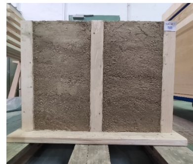
Figure 14. Top surface of a prototype geometrically identical to the one in Figure 13 but with a 32/68 sludge/aggregate ratio: only marginally more cracks recognizable
