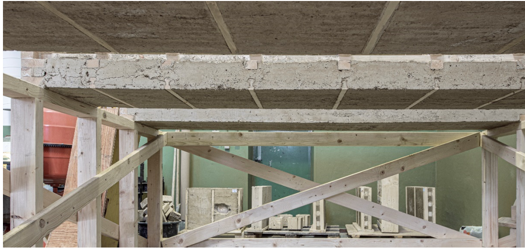
Figure 19. The finalized set of three M-series prototypes with earth infill.
