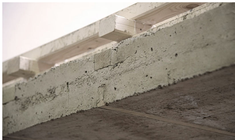
Figure 1. Side view of a 1:1 scale Timber Earth Slab prototype, showing how the layer of earth is located on the bottom of the slab and thus exposed towards the interior space.
