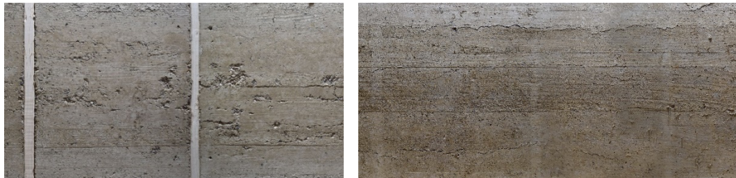
Figure 20. Surface excerpt from a prototype with coffering (left), showing a few shrinkage cracks in span direction but no tension cracks perpendicular to it, and without coffering (right), showing no tension cracks but an increased amount of shrinkage cracks parallel to the span direction. point of formwork removal and 10mm after 28 days of drying. This constant increase in bending can be explained by the continuous increase of humidity in the timber boards (see 4.4.2).
