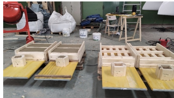
Figure 11. Casting studies of four geometrically identical S-prototypes to evaluate different earth mixtures with various water contents and sludge/aggregate ratios.
