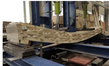
Figure 23. Four-point bending test.
