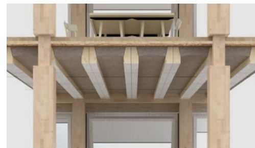
Figure 4. Model of the timber earth floor slab system; source: ZPF engineers and Herzog and de Meuron Architects.
