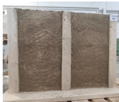
Figure 13. Top surface of the reference prototype: 60x40mm board format and a 24/76 sludge/aggregate ratio. Only very few and fine cracks are visible.
