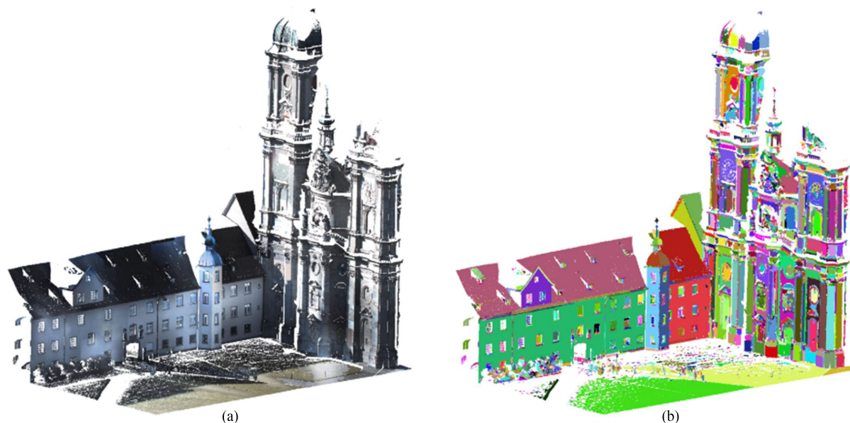
Fig. 14. Illustration of building segmentation. (a) Raw point cloud from TLS, rendered with RGB values and (b) segmentation results.
