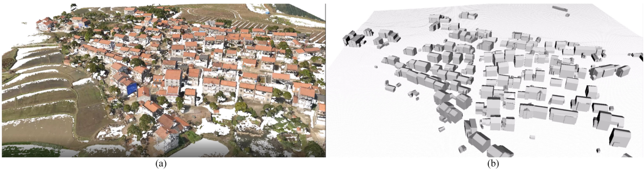
Fig. 20. Sketch of modeling of the point cloud. (a) Original photogrammetric point cloud from acquired by UAV. (b) Surface models of individual buildings.
