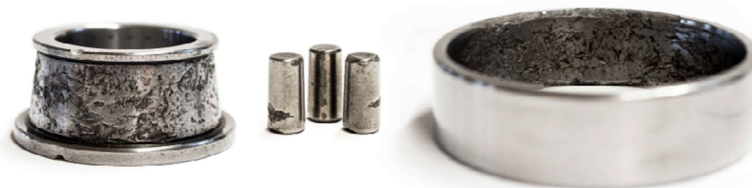
Figure 7. Faults in the accelerated wear tests, lower image following [7].
