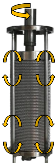
Figure 1.14. Image of catalyst basket with flow markers.
