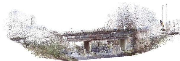
Figure 6: Original point cloud of bridge
