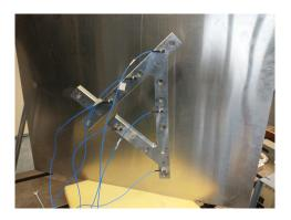
Figure 3.6: A-Frame with 6 Accelerometers.
