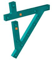
Figure 4.2: Mesh A-Frame Structure
