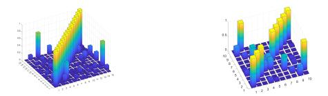
Figure 4.39: Experimental vs. Numerical MAC : A-Frame Figure 4.40: Experimental vs. Numerical MAC : Beam
