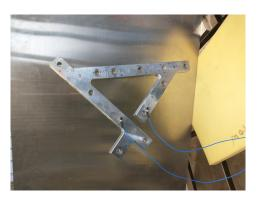
Figure 3.5: A-Frame with 2 Accelerometers.
