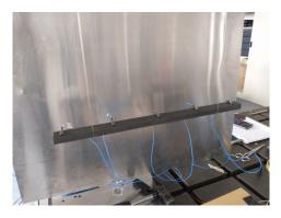
Figure 4.17: Beam 5 Accelerometer Setup
