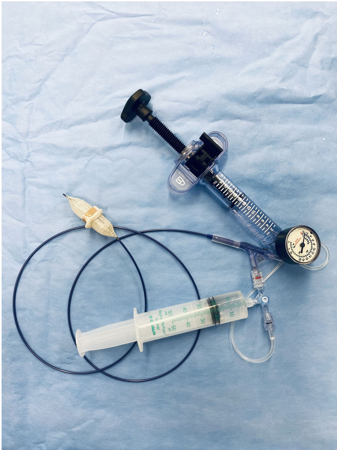
FIGURE 1 | In-vitro test setting with a high-pressure balloon connected via high-pressure stopcock to a 50-ml syringe containing dilute contrast and to a high-pressure inflator.
