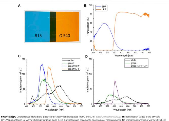
LPF. Values obtained via warm-white light emitting diode (LED) illumination and ocean optic spectrometer measurements. (**C**) Irradiation intensities of warm-white LED (SWW), green LED (510 nm), green LED with BPF and green LED with LPF at setpoint 200  $\mu$ mol m<sup>-2</sup> s<sup>-1</sup>. (**D**) Irradiation intensities of warm-white LED (SWW), green LED (510 nm) with BPF and LPF were set to 75  $\mu$ mol m<sup>-2</sup> s<sup>-1</sup>.
