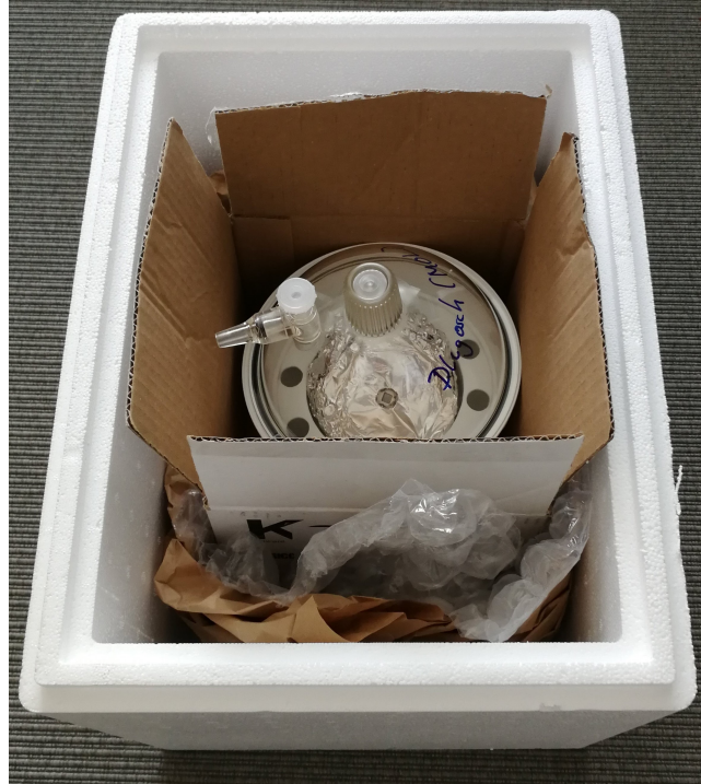
Figure 4.1.3 Shadow Mask Alignment kit transport box that was used to transport the aligned samples across the city. Styrofoam box serves the purpose of keeping the temperature inside the box as constant as possible, whereas the desiccator and the silica gel inside the evacuated desiccator were introduced to reduce humidity inside. Foil and paper were added to provide additional thermal isolation. This transport system aims to prevent condensation of water on the sample that might happen due to repeated temperature changes when moving from a warm to a cold and then to a warm environment again.
